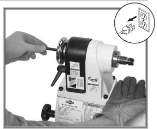
Figure 11. Removing spur center using knock out bar.
